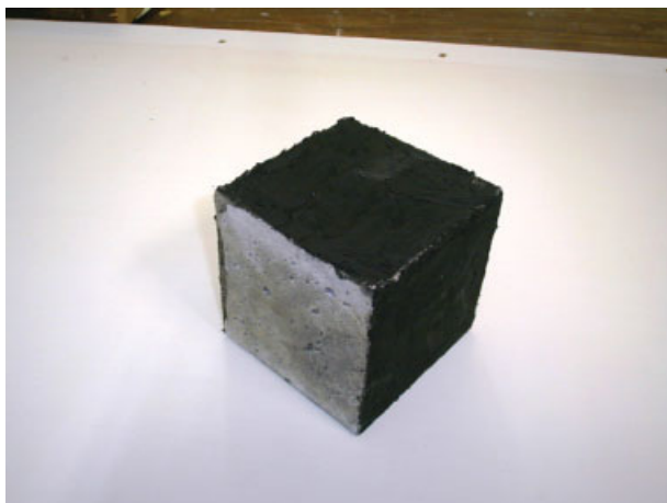
Figure 2 The cube mortar specimens with an epoxy resin paint. [Color figure can be viewed in the online issue, which is available at www.interscience.wiley.com .]
